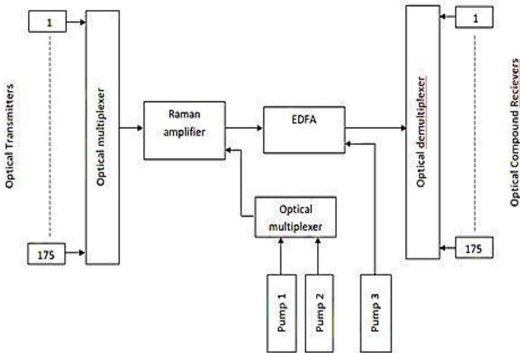
**Fig. 1:** Proposed block diagram of Hybrid Optical Amplifier.
