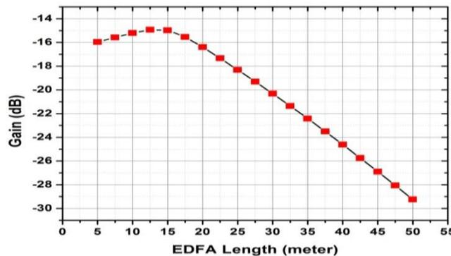
*Fig. 3: Gain spectra of HOA for different lengths of EDFA.*
