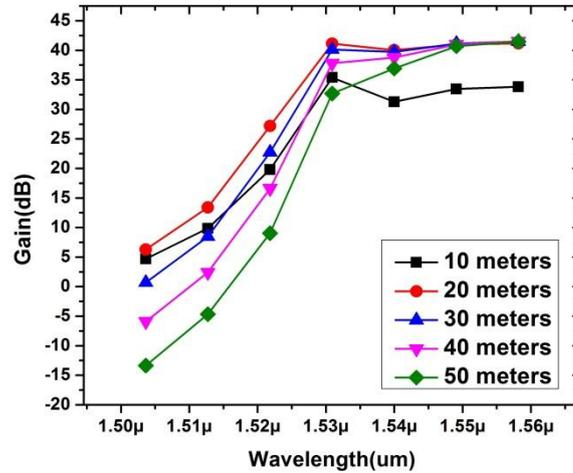
Fig. 4: Gain spectra of HOA for effect of different EDFA lengths at different wavelengths
