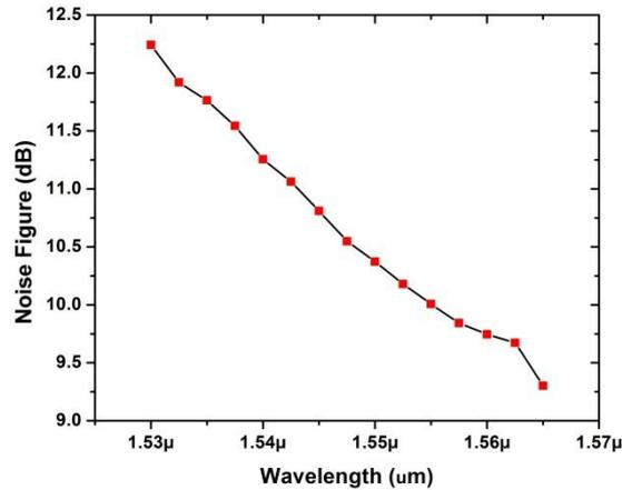
*Fig. 8: Effect of increment of wavelength on noise figure of the system.*
