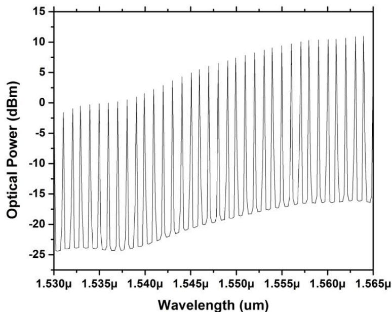
*Fig. 7: output optical spectrum of the DWDM system*
