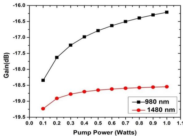
*Fig. 2: Gain spectra of HOA for different pump powers at 980 nm and 1480 nm pumping wavelengths of EDFA*
