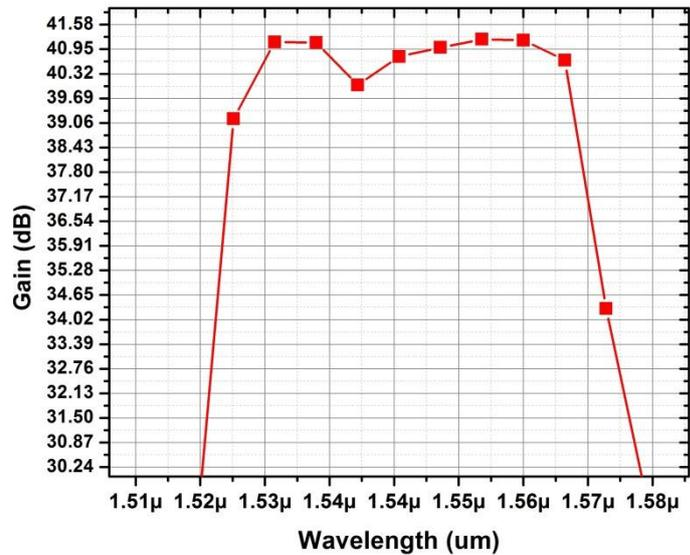
*Fig. 6: Gain spectra of HOA for different wavelength.*
