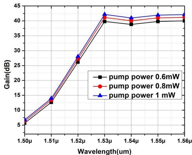
Fig. 5: Gain spectra of HOA for effect of different EDFA pump powers at different wavelengths
