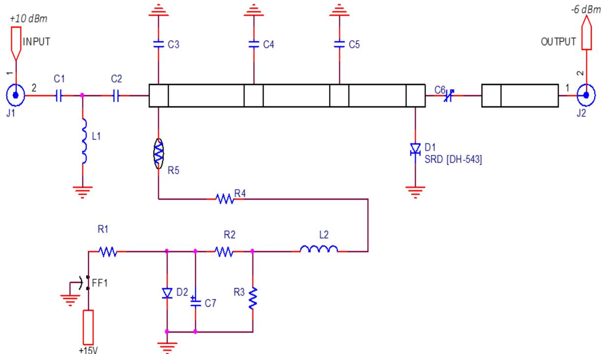
**Fig:2.** Schematic of X12 Frequency Multiplier
