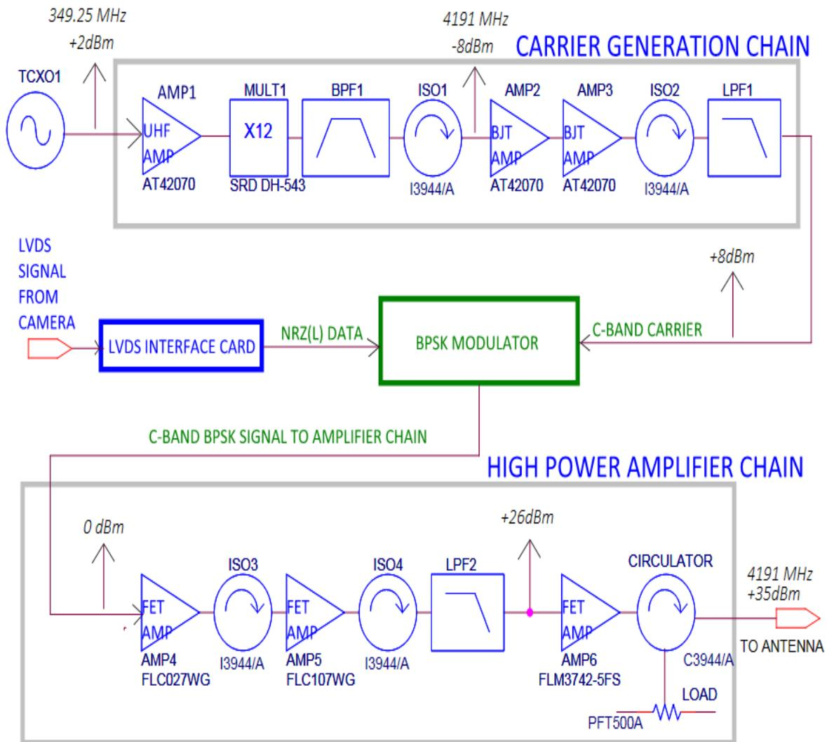
**Fig:1.** Block Level Schematic of C-Band Data Transmitter
