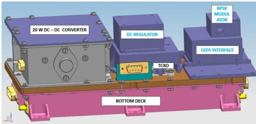
*Fig:3. 3D View of C-Band Data Transmitter*
