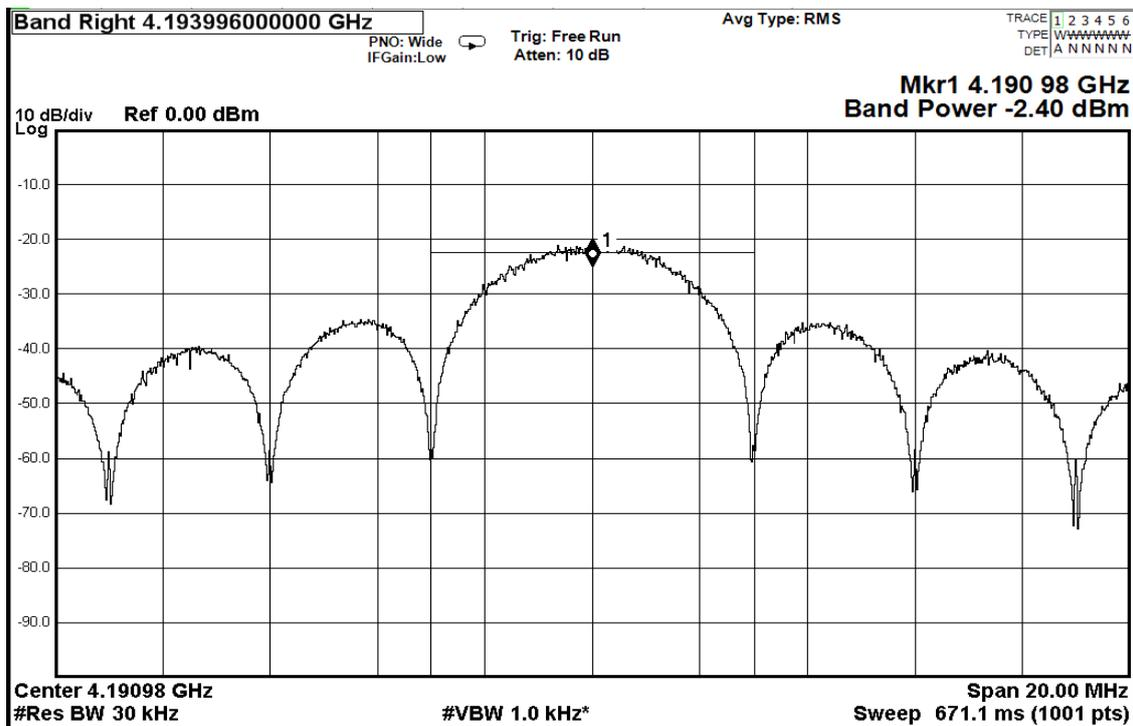
**Fig.5. Spectrum with PRBS Data Input**
