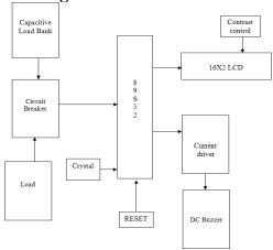
This the block diagram of the APFC panel. The supply to the circuit is applied from the regulated the power supply. The main supply is stepped down by the transformer to 12 volt and it is fed to the rectifier. The current and voltage signal are taken from the PT's and CT's. These two waveform are being change to the square wave through the zero crossing detector .Now
